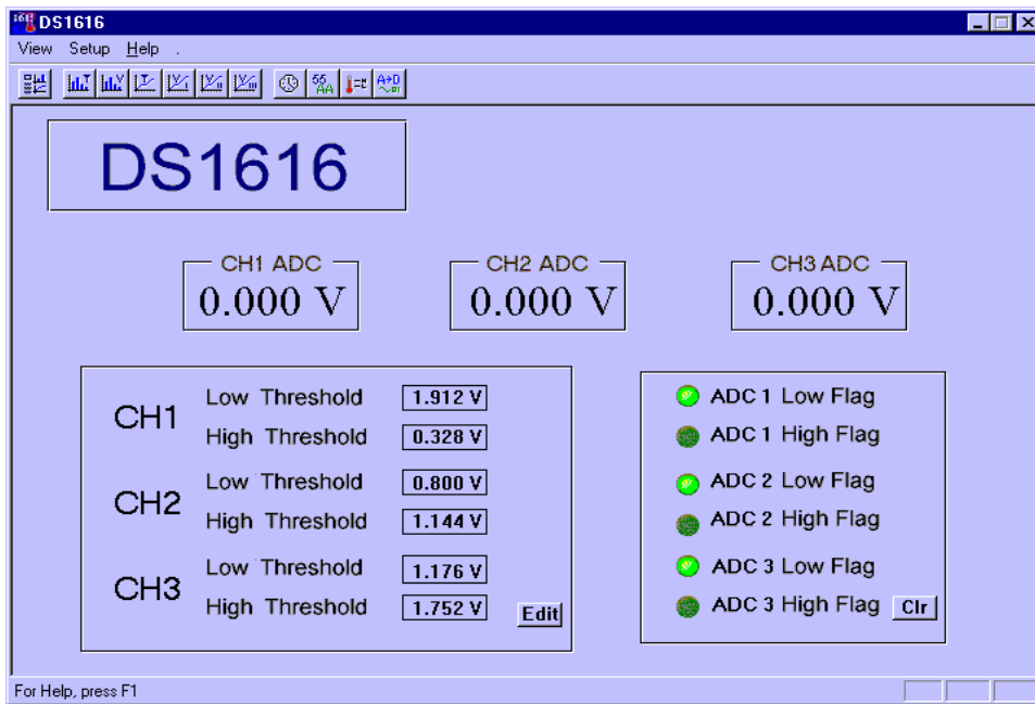
Figure 10: DS1616K ADC THRESHOLD SET MENU
